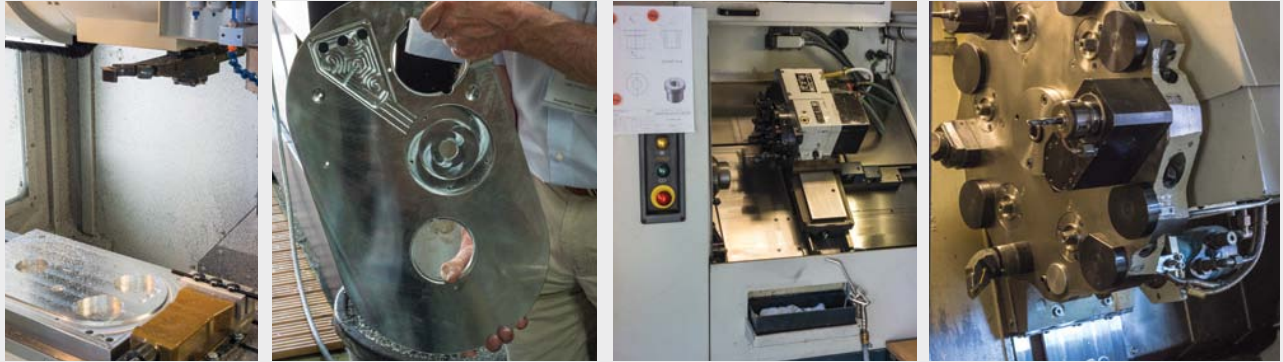
Photo 1 (far left), CNC machine milling V12 plinth. Photo 2 (left), finished V12 plinth. Photo 3 (right), computerized lathe. Photo 4 (far right), lathe fitted with bits to mill bearings.
