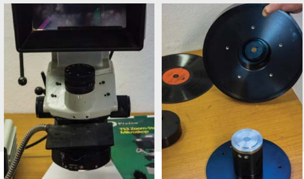
Photo 6 (bottom right), hydrodynamic turntable bearing.
