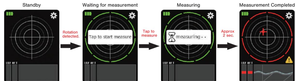
\*Please be sure to rotate the record player (33rpm or 45rpm) when measuring eccentricity. If the record player is not rotating, the stabilizer will not enter the measurement mode.
