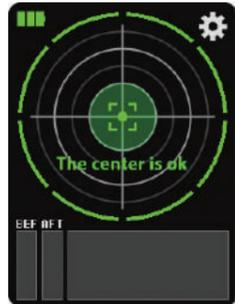
When the center of rotation is aligned with the absolute center position, rotate the record player again to check that the eccentricity of the record is gone (or reduced) and then play the record.
