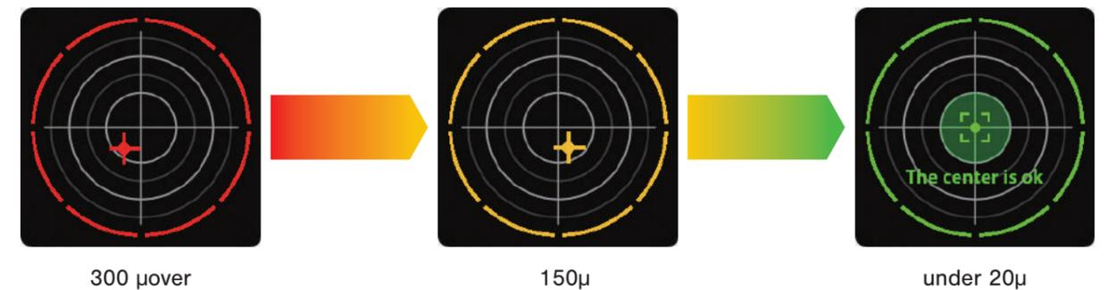
The color of the outer circumference, the cross mark, and the Before After display bar changes variably according to the amount of eccentricity.
