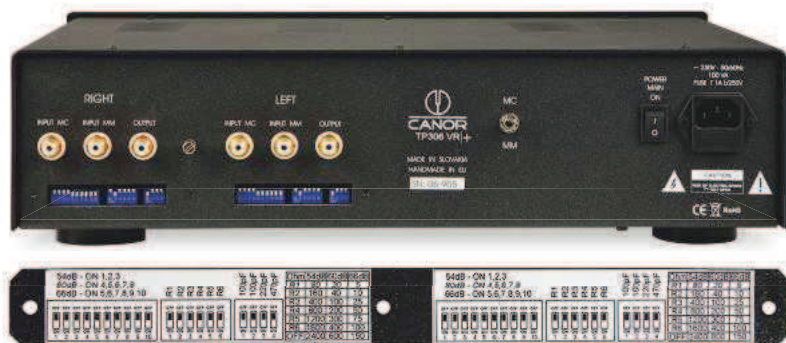
ABOVE: Rear panel layout reflects the dual-mono layout inside, while removing a small cover (shown enlarged) reveals DIP switches that give three gain settings and six load options for moving-coil, and capacitive loading for moving-magnet
