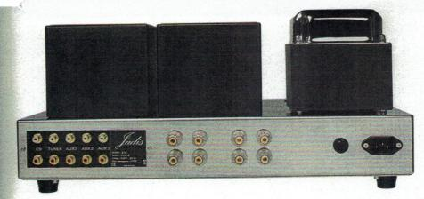
The left and right loudspeaker output sockets are paralleled, so give the same output.
